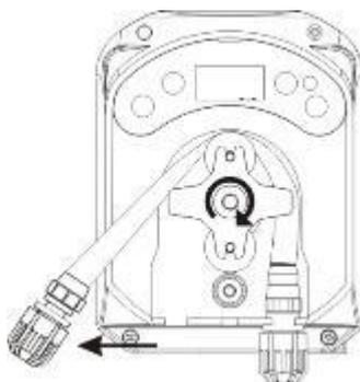
**Step 4** - Release t the (right) delivery ring nut and remove it completely
