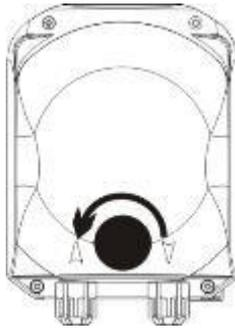
**Step 2**- Turn the roller clockwise and release the (left) intake ring nut
